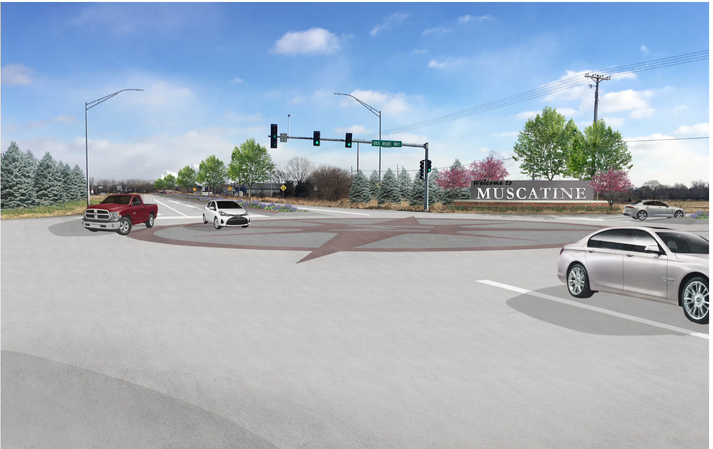
Figure 15: Design concept for focus site one. The perspective shows a signalized intersection with specialty paving, a new city of Muscatine welcome sign, landscaped medians, street trees, and evergreen tree screening to adjacent property owners.
