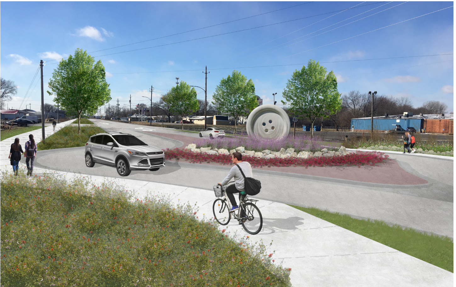
Figure 23: Design concept for focus site three. The perspective shows curved traffic lanes around the landscaped extra-large “eyebrow” median featuring a sculpture, trails on both sides of Grandview Avenue, street trees, stormwater swales with native plantings, and an upgraded Brier’s Ditch.
