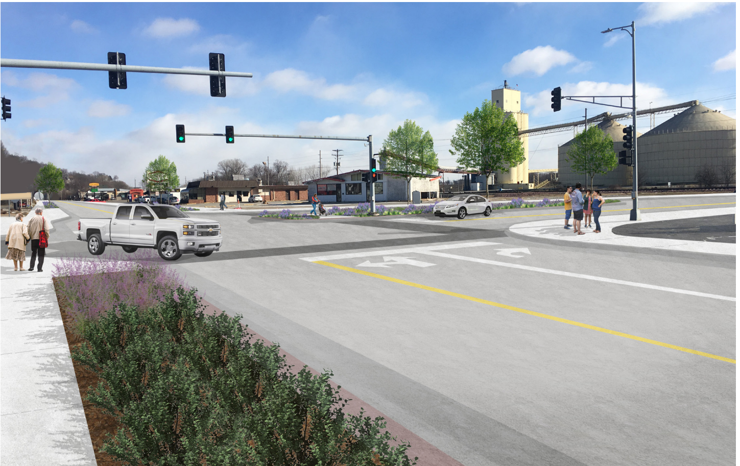
Figure 28: Design concept for focus site four. The perspective shows fewer travel lanes at this signalized intersection, stormwater landscaping on both sides of Grandview Avenue, a landscaped island at Oregon Street, pedestrian crosswalks, street trees, and a paver splash pad.
