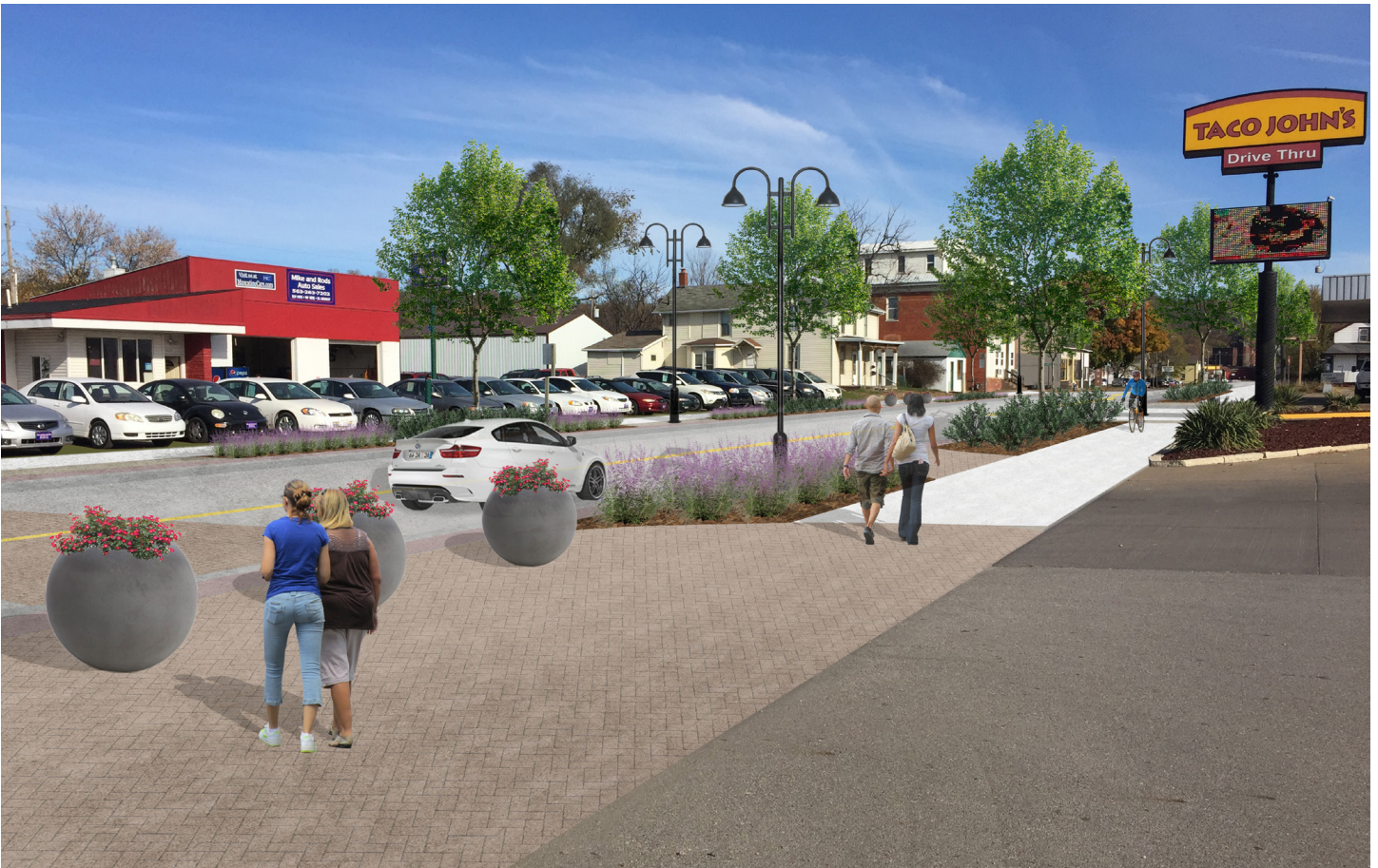
Figure 32: Design concept for focus site five. The perspective shows Grandview Avenue tapered to two-lane traffic, stormwater landscaping, street trees, special crosswalk paving, widened sidewalks, and decorative bollards and street lighting.
