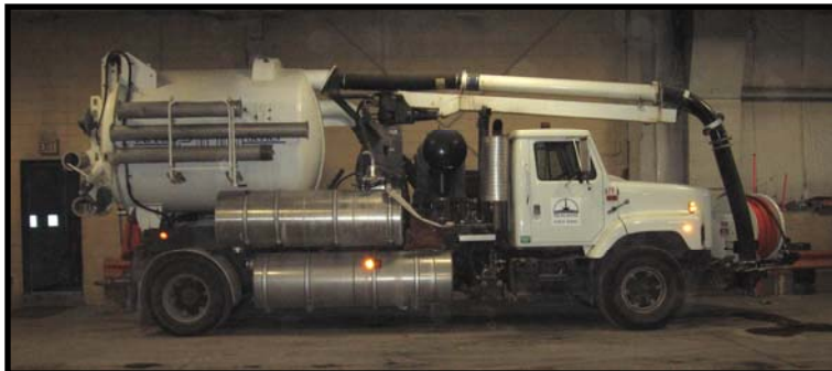
Jet Vac truck that is to be Replaced
